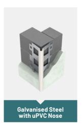
Manufactured with DX51D+Z galvanised steel strips with zinc coating of 275  $g/m^2$  on both sides in accordance to EN 10346 and protective uPVC nose. uPVC nose adds protection and a maintenance free finish.
